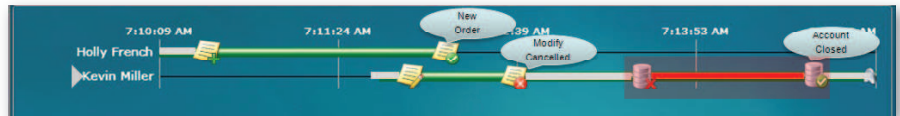
Desktop application screen event tags are graphically displayed as icons on a timeline of recorded interactions. Color indicates the type of activity between an initial and terminating event marker.
